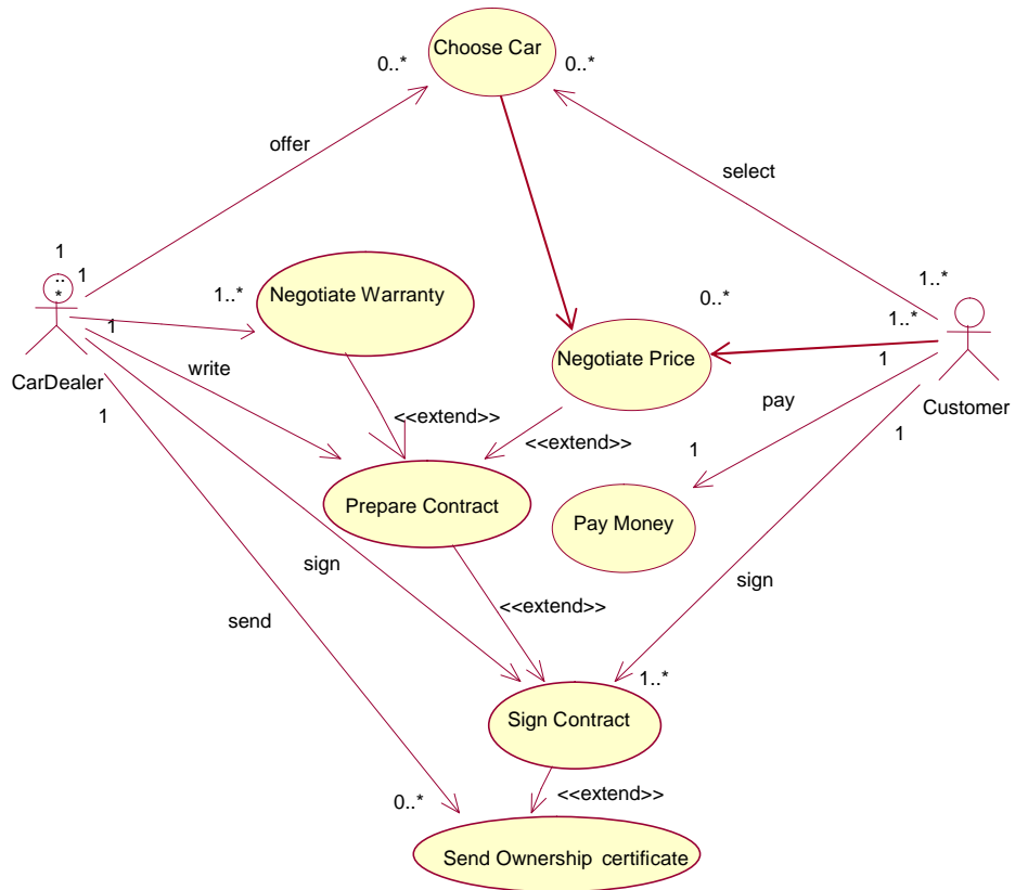
Figure 4. Use Case Diagram for the car example
