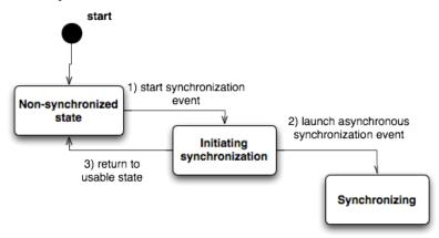
The Asynchronous Data Synchronization pattern is a mechanism pattern, thus it may be best visualized as a series of states. When an application is "usable" (meaning the user can interact with the application) a synchronization event can be started. Rather than executing the synchronization event sequentially, however, the event is launched asynchronously and the application returns to a usable state immediately.
