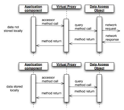
In the diagram, there are two sequences shown for two separate cases that encompass *Partial Storage*. First, the sequence is shown for when data needs to be accessed and is not stored on the device; second, the sequence is shown for when data is already stored on the device. This diagram uses other patterns described below in the solution section to help visualize the process using existing common patterns.
