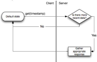
This flow chart shows the increased logic of a *Timestamp Transfer*. The client initiates a request and attaches a timestamp to the request, which is processed by the server to determine whether or not to return any data.
