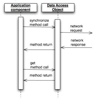
This sequence diagram gives a simplified version of *Complete Storage*. It draws a distinction between two types of actions: synchronization and a "get" action. The synchronization action causes a network request and returns data to
