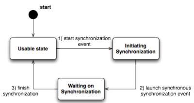
The Synchronous Data Synchronization pattern is a mechanism pattern as well, thus we will visualize it as a series of states. When an application is in a usable state, a synchronization event can be started. The event is launched synchronously and executed in a sequential fashion, leaving the application in a waiting state until the synchronization is finished, whereupon it returns to the usable state.
